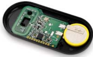
m130 Active RFID asset tag from RF Code
