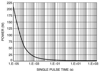
Figure 12. Single Pulse Maximum Power Dissipation
