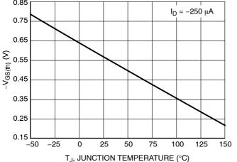
Figure 11. Threshold Voltage
