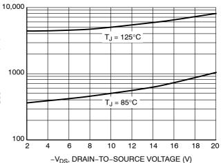
Figure 5. On–Resistance Variation with Temperature
