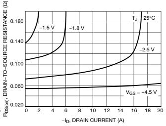
Figure 3. On-Resistance vs. Gate-to-Source Voltage
